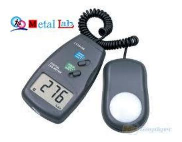
The digital lux meter LX1010B can measure up to 50,000 lux, approximately 5,000 foot candles. It's used for checking the level of luminance, luminance is a measure of the amount of light falling on a surface. It is defined as: 'the density of the luminous flux incident on a surface'. It is the quotient of the luminous flux by the area of the surface when the latter is uniformly illuminated. This convenient gadget is widely used in many areas such as construction, inspection, photography and etc.
